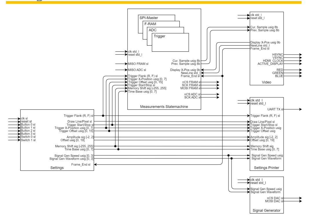
The design incorporates a modular and robust system featuring ADC inputs, a video generator for display output, external F-RAM for signal buffering, and UART for configuration monitoring. It achieves VGA-compatible output with a rotated display to minimize memory usage and includes a versatile test signal generator alongside real-time setting adjustments.
