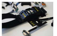
Figure 13: Modular wearable biosignal measurement platform
